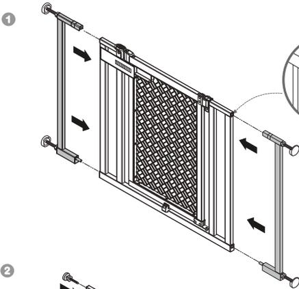
Connect the extension frames to gate frame by inserting the pins on the extension frames into the holes in the gate frame.
