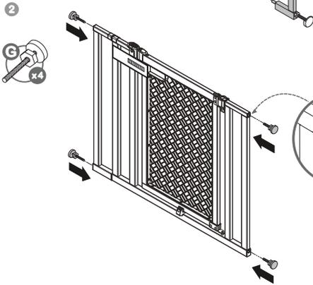
Slide tension bolts into upper and lower holes on both sides of the gate assembly. The holes are not threaded and that the tension bolts should slide freely.
