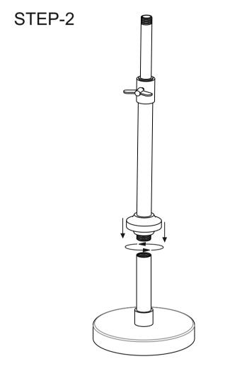
Now insert middle post on top of bottom post and secure it, as shown.
