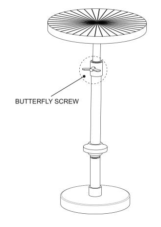
To adjust height of table, loosen butterfly screw, position inner post to desired height and retighten butterfly screw.
