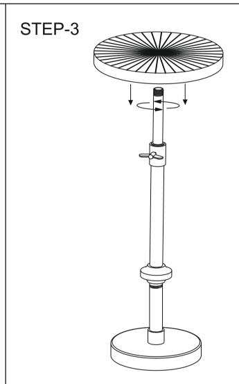
Fix Table top to the top of inserted pipe.
