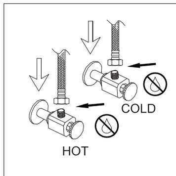
5. Connect hoses to the water supply and tighten. Check all connections at arrows for leaks. Retighten if necessary, but do not overtighten.
