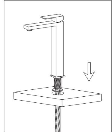
2. Install faucet with oring under the flange through center hole.
