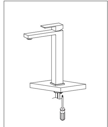
4. Hand tighten further using a screw driver to tighten lock nut screws.
