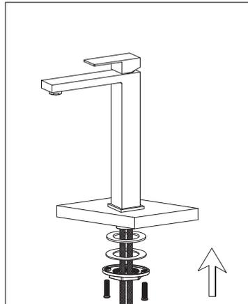
3. Re-install the rubber washer followed by the metal washer and lock nut, then hand tighten it.
