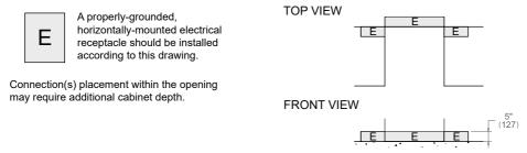
Dimensions in parentheses are millimeters unless otherwise specified.
