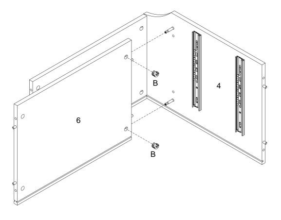
Using Cam lock(B) secure part (6) to part (4) with Philips head screwdriver as per diagram.
