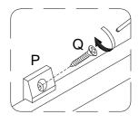
Using screw (Q) secure plastic wedge (P) to parts (5,7) with Philips head screwdriver as per diagram.
