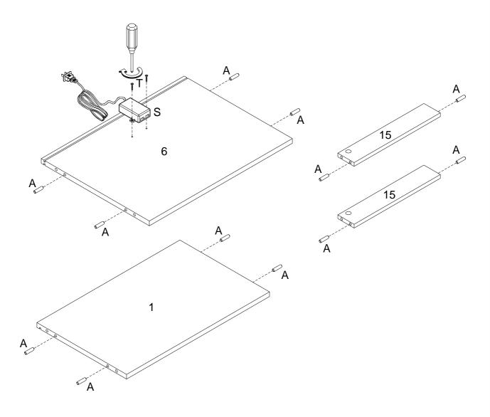
Insert wooden dowel (A) into parts (1,6,15), using screw (T) attach USB interface to part (6) with Philips head screwdriver as per diagram.
