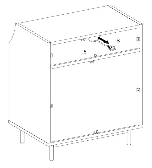
Take out the plug (S) from the core management hole as per diagram.
