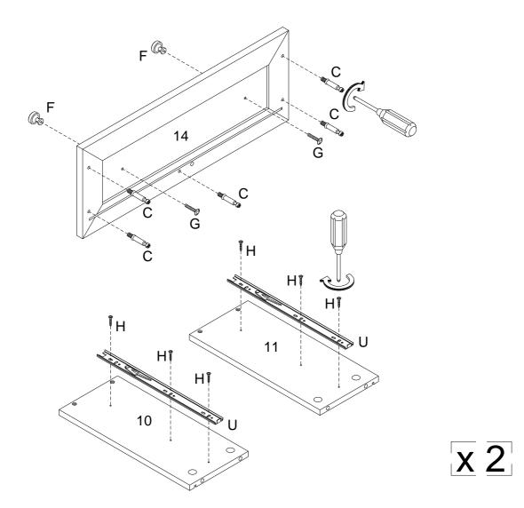
Secure Cam bolt (C) into part (14) ,then using handle bolt (G) secure handle (F) to part (14) and using screw (H) attach drawer slider (U) to parts (10,11) with Philips head screwdriver as per diagram.
