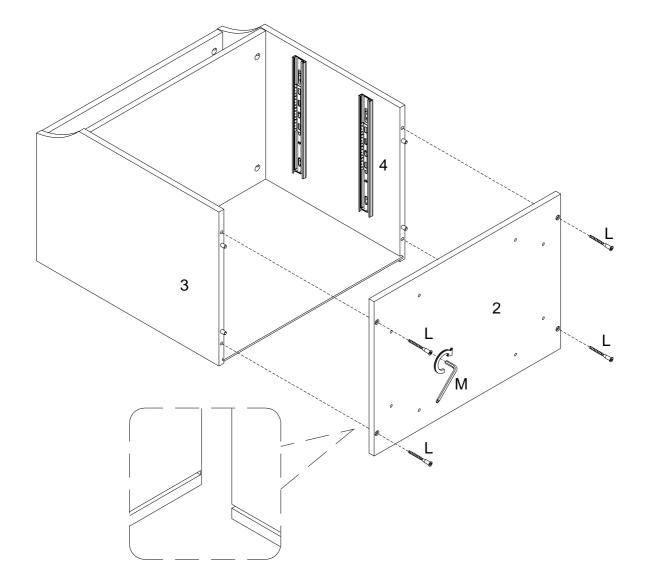
Using screw (L) attach part (2) into parts (3,4) with Hex key (M) as per diagram.
