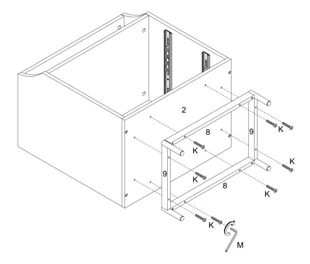
Using bolt (K) attach parts (8,9) to part (2) with Hex key (M) as per diagram.
