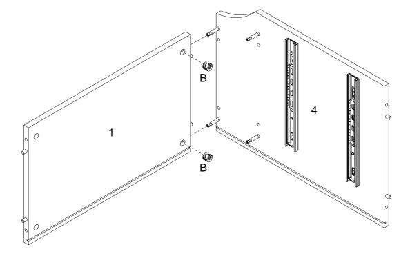
Using Cam lock(B) secure part (1) to part (4) with Philips head screwdriver as per diagram.
