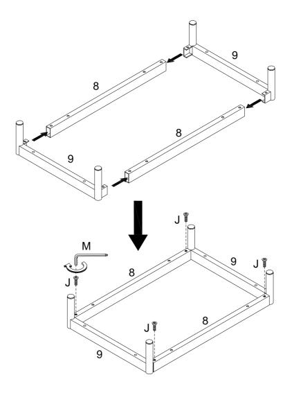
Attach parts (9) into part (8) ,then using bolt (J) secure part (8) to part (9) with hex key (M) as per diagram.
