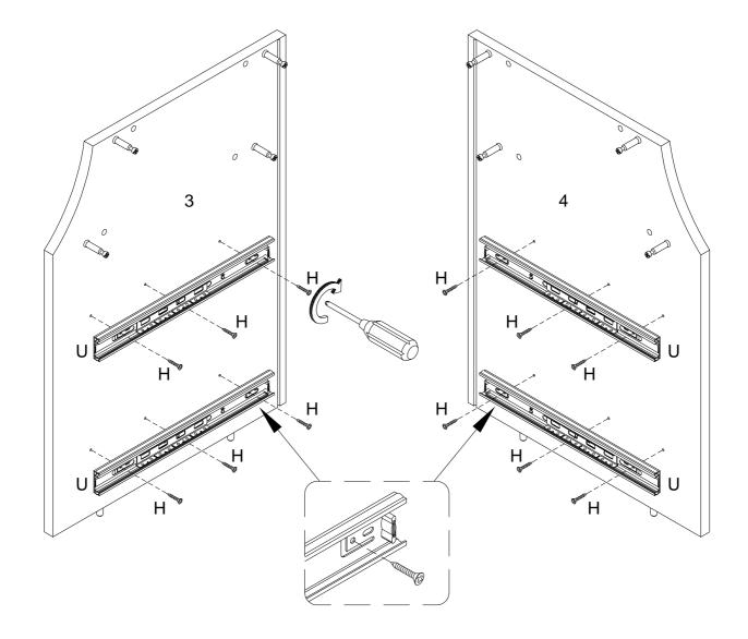
Using screw (H) attach drawer slider (U) to parts (3,4) with Philips head screwdriver as per diagram.
