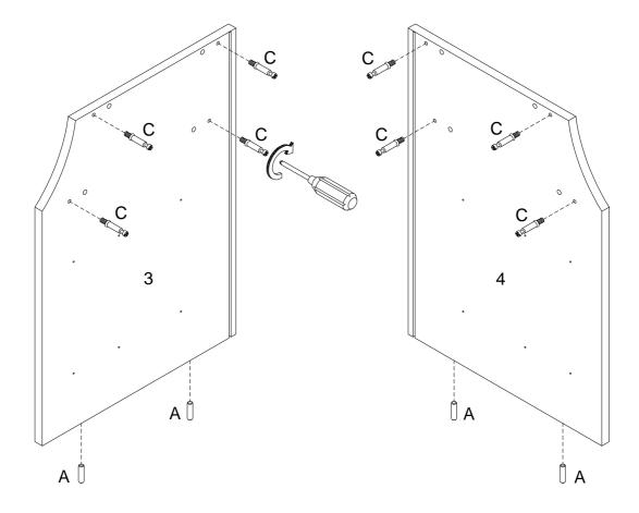
Insert wooden dowel (A) into parts (3,4), and secure Cam bolt (C) into parts (3,4) with Philips head screwdriver as per diagram.
