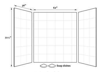
Designed to fit base areas 36" deep or smaller x 62" wide x 72" high or smaller (914 mm x 1575 mm x 1829 mm)
