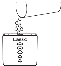
2. Add water to the Tank. Be sure to always use Distilled Water. DO NOT PUT BOILING WATER IN UNIT.
