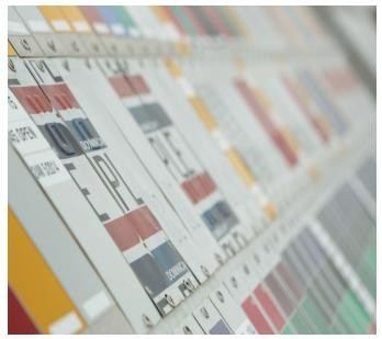
3M performs weathering tests on many of our products using the most advanced weather facilities in the world. Substrates bonded with 3M VHB Tape are subjected to artificial indoor tests and real-world outdoor tests to determine the effects of years of extreme weathering. Exposing them to extreme UV radiation, water and heat ensures your products can stand the test of time.
