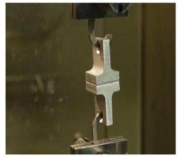
Dynamic normal tensile test: Quantifies the internal cohesive strength of 3M VHB Tape. Unlike mechanical fasteners, the viscoelastic foam core of 3M VHB Tape absorbs the tensile stress, spreading the stress throughout the entire bond.
