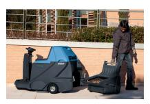
Emptying the 65-liter debris hopper is a breeze thanks to its equipped wheels, simplifying the task and minimizing downtime.
