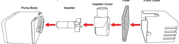
Press down on the top of the front cover and pulling it off by the sides.
