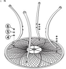
Loosely fasten each leg to the tabletop using Flat Washer (4), Split Washer (5), and Nut (6).
