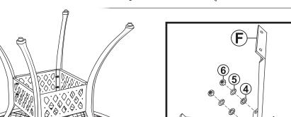
Fasten the four Panels (F) to the legs using Flat Washers (4), Split Washers (5), and Nuts (6).
