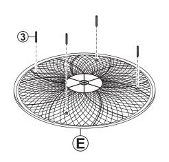
Place Tabletop (E) face down on a soft, clean surface. Firmly secure four Grub Screws (3) to the table top.
