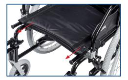
From the underside of the seat, pull down and away seat upholstery flap to free up seat extension. Pull outward on the fastener strips to free from upholstery.
