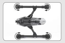
Having confirmed that all works as it should and that the motors rotate correctly, disconnect the battery and switch OFF your transmitter. Identify the propellers noting that two of the four have a right-hand rotation (denoted by the letter R alongside the dimension embossed on the root section of the blade). R designated propellers should be
