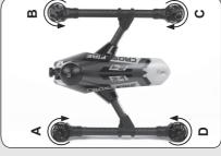
installed on motors A and C and fitted with a black (left-hand thread) prop nut. The remaining left-hand rotation propellers should be secured to motors B and D.
