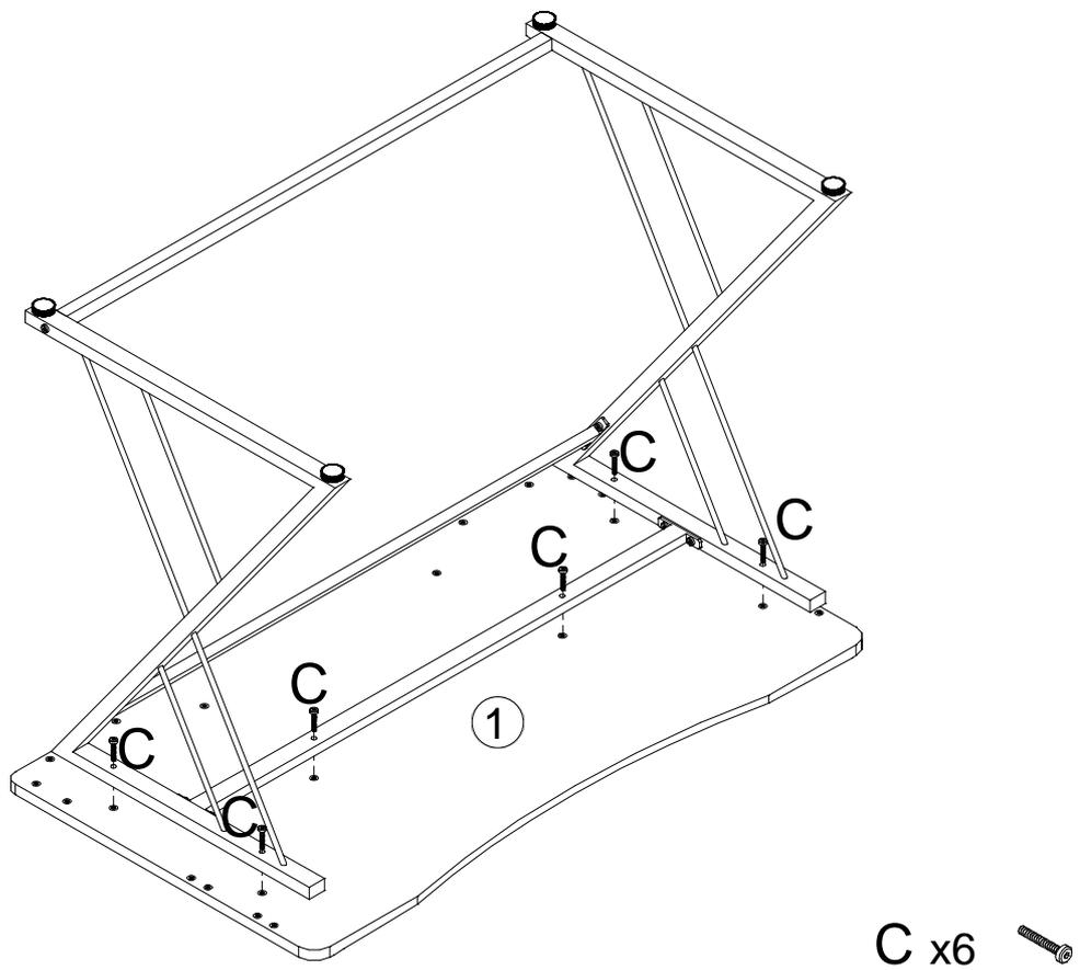
Note: Please keep the iron frame perpendicular to the back of the board
