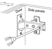
In-and-Out by loosening the hinge-arm mounting screw or via cam adjustment
