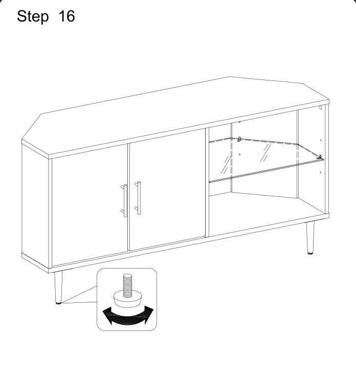
Position the assembled unit at the deaired location. If necessary adjust the floor levelers at the bottom of legs to level the unit .
