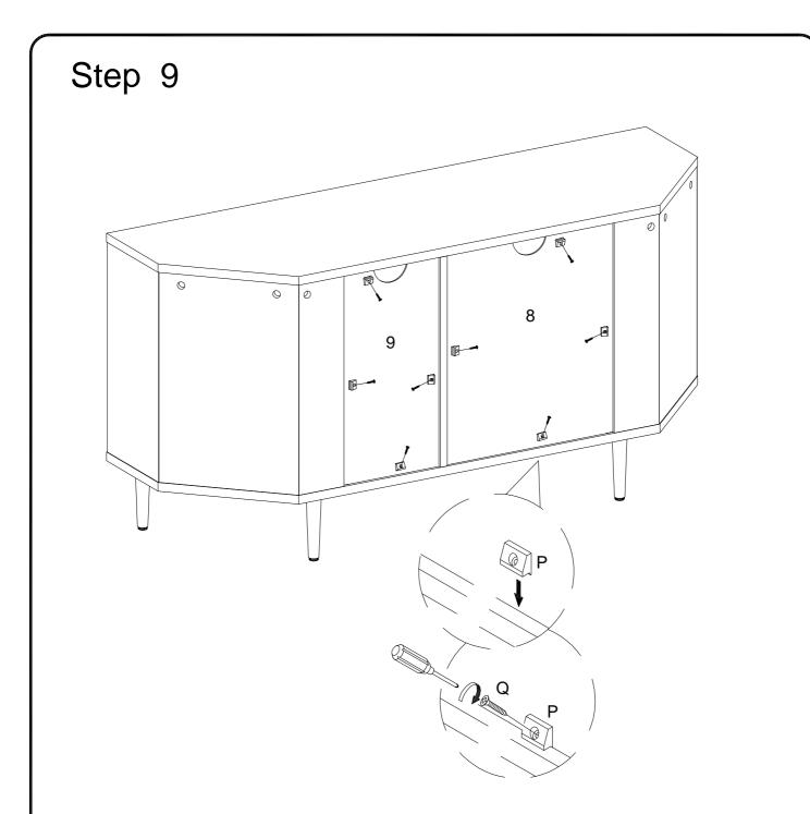
Using screw (Q) secure plastic wedge (P) to fix parts (8,9) with Philips head screwdriver as per diagram .
