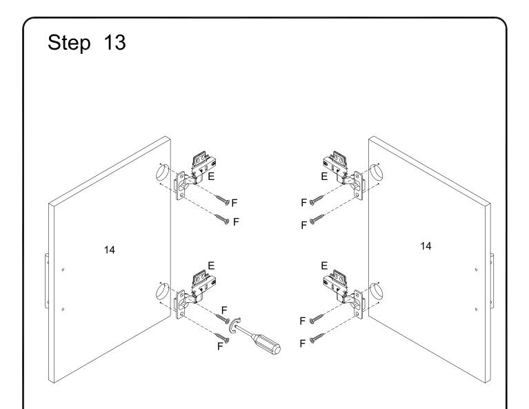
Using screw (F) attach Europe hinge (E) into part (14) with Philips head screwdriver as per diagram.
