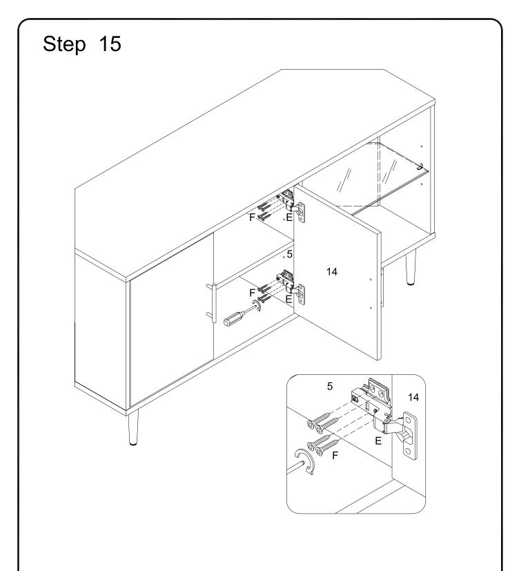
Using screw (F) attach Europe (E) into part (5) with Philips head screwdriver as per diagram. Close and open the doors to make sure they are shut correctly .If necessary ,adjust the screws (F) for a good fit .
