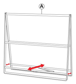
Pull the bottom of Stand (A) outward until it is fully extended.
