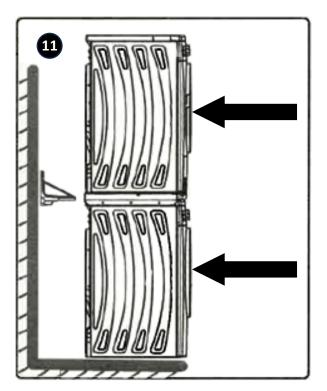
Step 11: With assistance, slide the stacked washer and dryer back against the wall, allowing the wall bracket to hold the assembly in place.
