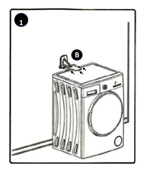
Step 1: Position the washer against the wall where it be installed. Place the wall bracket on top of the washer and slide back until the flat rear of the bracket is flush to the wall.
