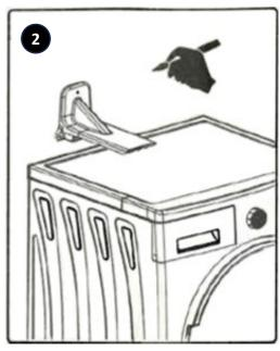
Step 2: Mark the position of the holes in the bracket on the wall with a pencil.
