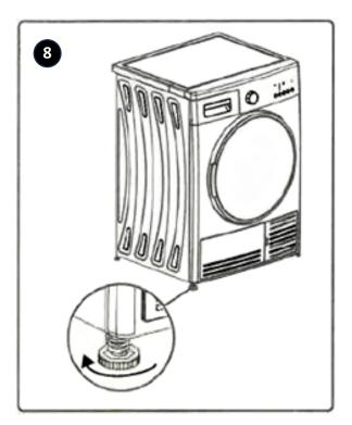
Step 8: Turn the leveling feet on the dryer all the way in to the lowest setting.
