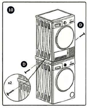
Step 10: Use 2 screws to secure the dryer to the stacking bracket.
