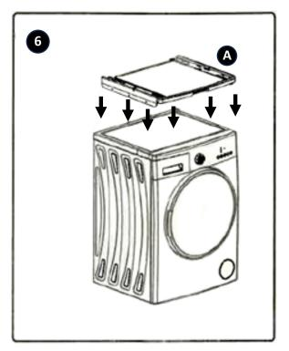
Step 6: Place the stacking bracket on top of the washing machine.
