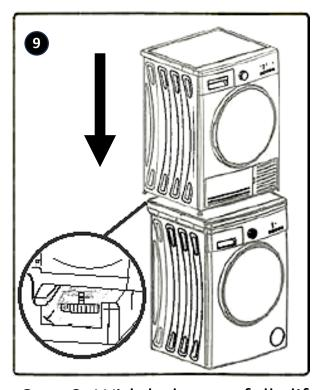
Step 9: With help, carefully lift the dryer on top of the stacking bracket. Slide the leveling legs into the support grooves in the bracket. Make sure the dryer is square with the washing machine
