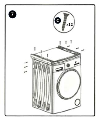
Step 7: Use the twelve (12) screws to secure the bracket to the top of the washing machine.
