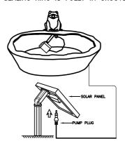
7. INSERT THE SPIKE INTO THE GROUND. POSITION THE SOLAR PANEL TO FACE SOUTH (In Northern Hemisphere) AS MUCH AS POSSIBLE TO MAKE THE MOST OF THE DAYLIGHT HOURS. IT IS IMPORTANT TO ANGLE THE SOLAR PANEL TO FACE SUN WHEN SUN IS AT ITS HIGHEST POINT. ENSURE THE SOLAR PANEL IS NOT SHADED BY TREES, SHRUBS OR BUILDINGS.
