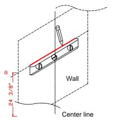
Step 2: Draw a horizontal line from the point a by using a leveler. (suggested H24 3/8" from floor to "a" line)
