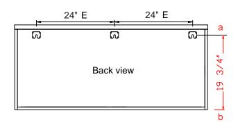
Step 1: Metal plates has been pre-installed to the back of cabinet, measure the distance between the bottom of the cabinet and point a.
