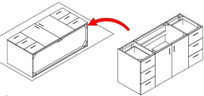
Step 1: To attach the metal legs, place the cabinet lay down on a blanket or similar soft material.
