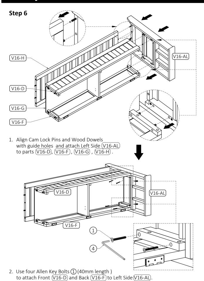
3. Use Allen Key (4) to tighten Bolts. Do not over-tighten.
