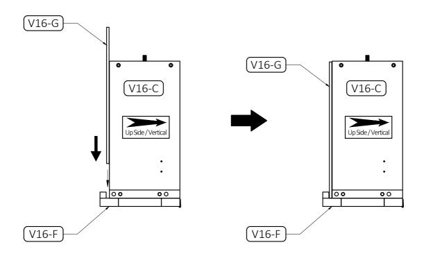
1. Attach Bottom Panel (V16-G) to Divider (V16-C) & Back (V16-F) by sliding on the gap between Divider (V16-C) & the long rail on Back (V16-F).
