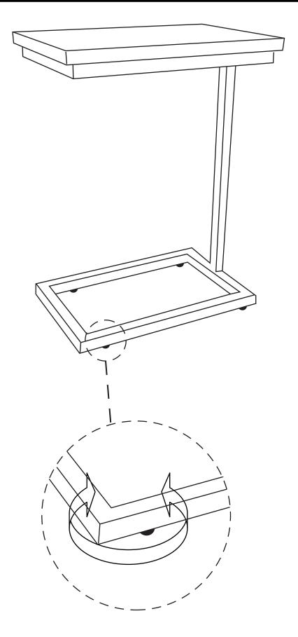
Note: Levelers underneath the base can be adjusted if floor is uneven.
