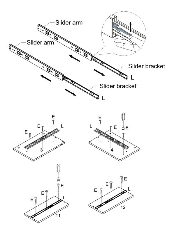
Separate the slider arm (L) using trigger , using screw (E) secure slider arm (L) to parts (3,4,11,12) as per diagram.
