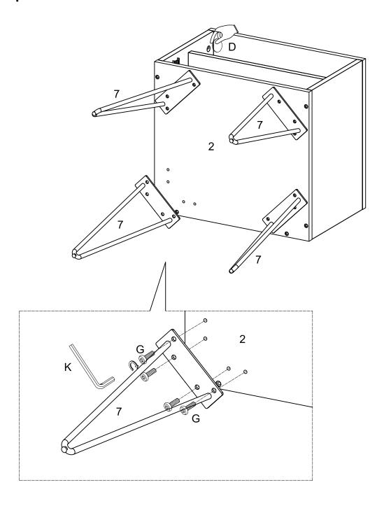
Using bolt (G) secure part (7) to part (20 with hex key (K) ,then using sticker (D) cover the hole as per diagram.
