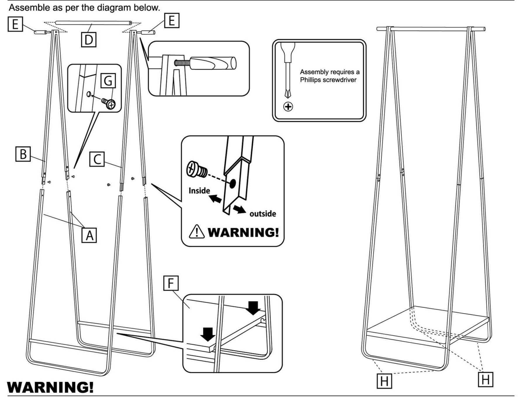
Max loading weight (bar×10lbs%5kg) (Side hook×2lbs%1kgs) (Shelf×10lbs%5kg)
