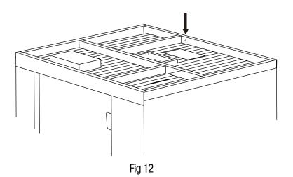
12. Put the Duster cover [1] on the Top board, then fix the Duster cover with self-tapping screws (3\*25) at the four corners. (Fig 13)
