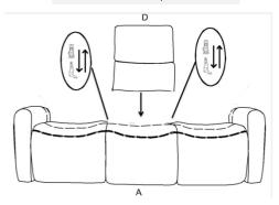
STEP 1 - Place Bracket into Sleeve and presstop of back down firmly to lock your KD back in place
