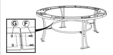
Loosely fasten the sides of the shelves using two Bolts (F) and Nuts (G).
