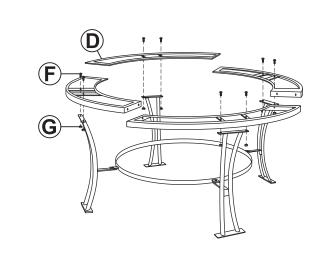
Loosely fasten one Shelf (D) onto each leg using two Bolts (F) and Nuts (G).
