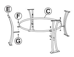
Loosely fasten Support Ring (C) onto Legs (E) using Bolts (F) and Nuts (G).
