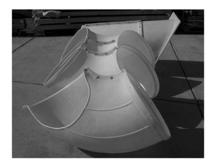
Connect the flanges of each tube section to make 3 elbows. Use 7/8" Hex Head Machine Bolts in 3 holes. In the fourth hole (the hole closest to female end), use a 1" Hex Head Machine bolt. Place a washer on each side with a 5/16" Loc nut to secure the bolts. Repeat this step for the straight tube. **Do not tighten bolts at this time.**
