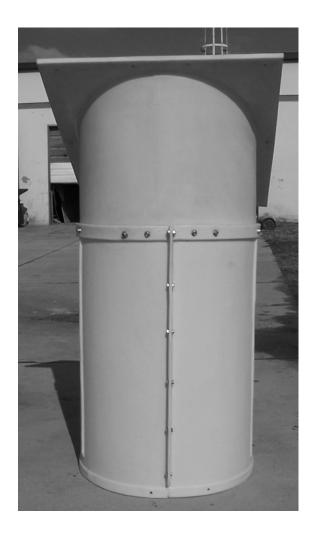
Stand up the Straight Tube with the female end up and insert the Mounting Tube. (You may need to temporarily remove the end bolt in the flange) Align the flange of the Straight Tube and the seam on the <u>long side</u> of the Mounting Tube. Tighten the bolts in the flange to hold the sections in place.
