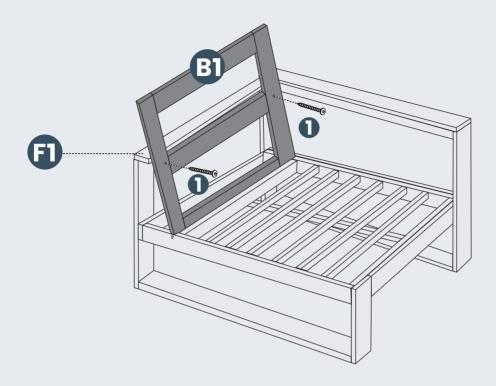
Check and tighten all the screws when the parts are loosely attached.
