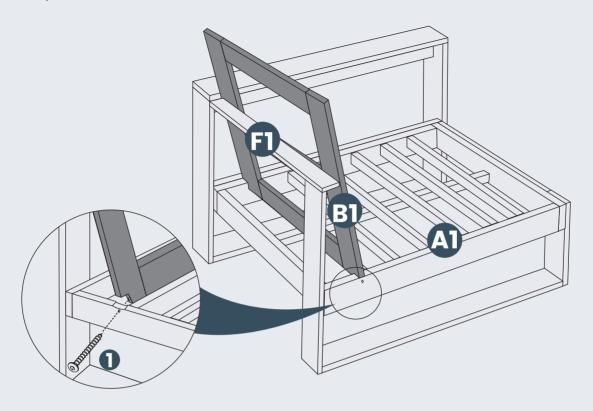
Attach Part Bl Backrest to Part Gl Chair Left Arm with 1 pc of Hardware #2 Screw.
