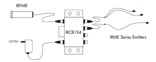
Drill a hole 7/16" diameter (10mm) wide where you wish to position the IR Receiver. Remove the screw-nut, push the receiver cable and through the hole with the lens facing into the room (and in line-of-sight of your hand-held remote). Screw the nut back on until tight to hold the IR Receiver in place.
