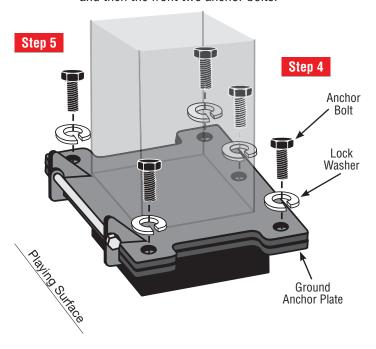
**Step 6:** Snug tighten the five anchor bolts, then check goal assembly with a level and inspect visually to determine if it is parallel and plumb to the playing surface.
