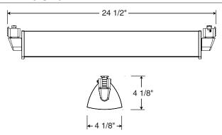
**Alternate HTYPE Trac Adapter** Compatible with track systems which use a H-type track adapter, including Lithonia LTS Decorative Track (not LT type) • System specific and assembled to trac fixture
