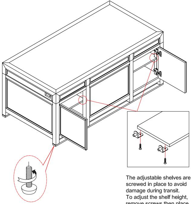
Adjust Leveler if needed to level Desk on uneven floor.
