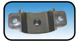
Step 9 The drain saddle must be mounted at least 1 ½” above the nut of the P-trap or cross bar from the garbage disposal to insure proper drainage. Assemble the drain saddle around the drain pipe at the best available location. Using Phillips screw driver tighten screws evenly and securely on both sides of the drain saddle. Keep the plastic compression nut off at this time.
