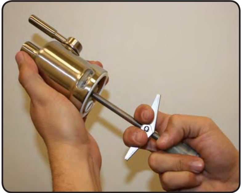
Disassembling your faucet is never recommended as this could void your warranty. If it is necessary to remove the fitting at the end of the toggle bolt you must follow the following procedure for re-assembly. Prior to re-connecting the fitting to the toggle bolt, you must insert the 3/8" blue tube into the fitting. There are small O-rings inside of the fitting that could be pushed out of position if the blue tube is not fully inserted first. Failure to do so may cause the faucet to leak.
