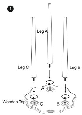
Keep the wooden top on clean surface as shown in the fig. Following the direction arrows marked on top and legs, place the legs (A,B,C) with corresponding grooves marked (A,B,C) on the wooden top. Now tighten the legs onto the fasteners provided on the bottom of wooden top as shown.
