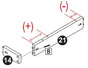
Identify the two indents on Center Drawer Rail (21), the indent with the longer distance between the indent and the edge of the rail must be installed toward Drawer Rail Support (14).
