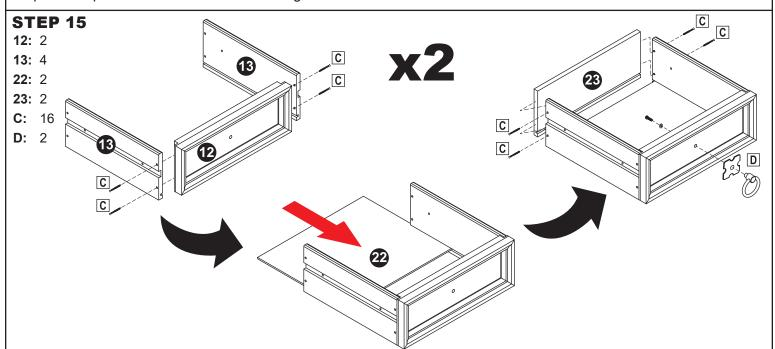
Ensuring the inside grooves align, secure two Drawer Sides (13) to Drawer Face (12) using four M3.5x30mm Flat Screws (C).
