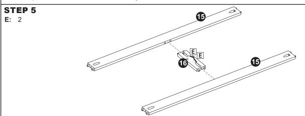
With the angled mounting holes facing upward, align two Horizontal Face Frames (15) and Vertical Face Frame (16). Secure using two M3.5x25mm Pan Screws (E).
