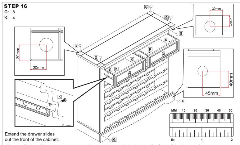
Align the first small hole on the drawer slides with the pre-drilled hole on the front of the drawer sides.
