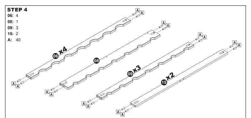
Install four Wood Dowels (A) into four Back Bottle Rails (06), Front Base Bottle Rail (08), three Front Bottle Rails (09), and two Horizontal Face Frames (15), as shown.
