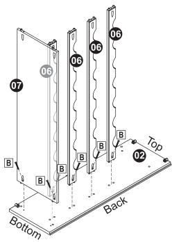
Ensuring the angled mounting holes face the back and the wine bottle grooves face the top, align four Back Bottle Rails (06) with Left Side Panel (02) and secure using four M4.5x28mm Pan Screws (B).
