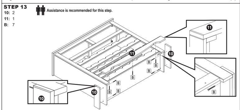
**NOTE:** Have an assistant firmly hold the trim boards in place to ensure they remain flush with the unit while hardware is secured.
