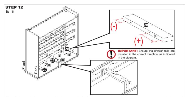
Identify the two indents on Outside Drawer Rails (20), the indent with the shortest distance between the indent and the edge of the rail must be installed toward the <u>front</u> of the cabinet.
