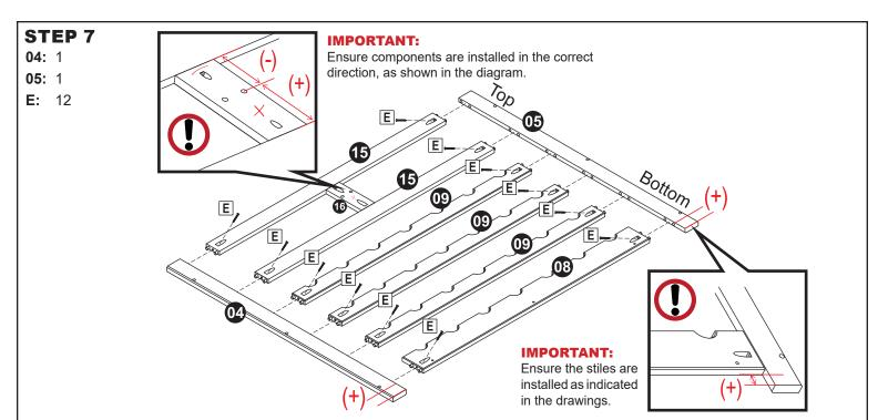
With the angled mounting holes facing upward, lay out the assembled face frame (15,16,15), three Front Bottle Rails (09), Front Base Bottle Rail (08), Right Stile (04), and Left Stile (05), as shown above.
