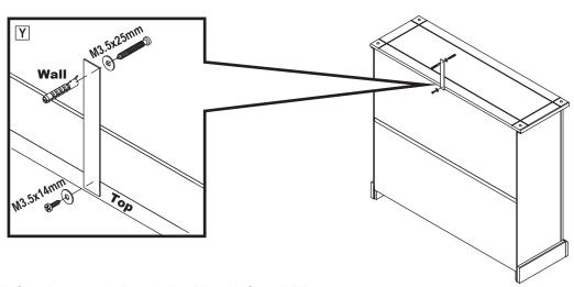
**WARNING:** Check for pipes and electrical wiring before drilling.
