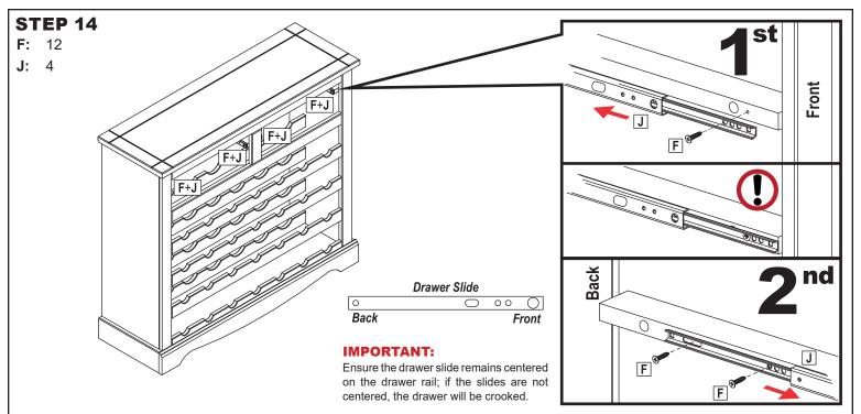
Push the front of Drawer Slide (J) backward. Align the 3rd round hole on the front of the drawer slide with the front indent on the drawer rail and secure using one M4x14mm Flat Screw (F).
