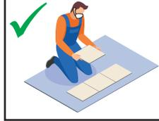
**TIP:** Use the box carton as a protective layer to separate and protect the parts from scratches and other damage during assembly.
