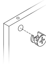
Align the cam lock opening (arrow) with the pre-drilled hole on the side of the panel. Use a screwdriver to adjust alignment as needed.
