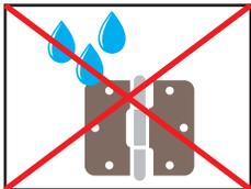
Do not allow metal components to come in contact with water or cleaners as it may cause rust and staining.
