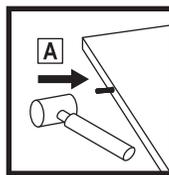
**TIP:** Install wood dowels by gently tapping them into the designated hole using a rubber mallet.
