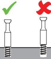
Use a screwdriver to tighten the cam screw until the shoulder is flush with the panel. Do not over-tighten or under-tighten.
