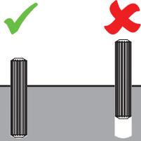
Install wood dowels by gently tapping them into the designated hole using a rubber mallet.
