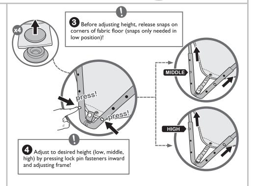
**IMPORTANT:** Ensure lock pin fasteners are properly engaged (8 places). All fasteners must be adjusted to the same position. Relock frame (2 places).
