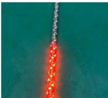
#1.Top section of LEDs are not bright
