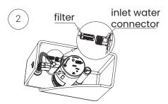
Remove the filter screen from the inlet water connector.
