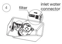
Re-install clean filter back into water connector
