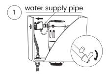
Shut off the water supply valve, then remove the water supply pipe.
