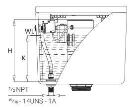
H: adjustable height:  $10^{5}/_{16}$ " -  $12^{3}/_{16}$ " K: adjustable height:  $6^{1}/_{2}$ " -  $9^{13}/_{16}$ " Adjustments include the height of the 8mm rubber gasket.
