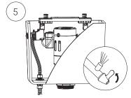
Insert the water supply pipe back to the water connector and turn on the water supply valve.
