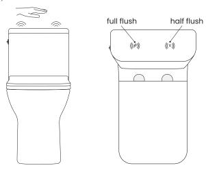
**NOTE:** If something is sensor recognized on the lid of the water tank, the toilet comes with an adaptive function, and will wait 30 seconds to resume normal use to prevent accidental flushing.
