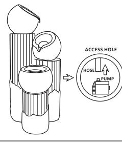
**2.** Extend the pump and LED light cables through the access hole in the back of the fountain, cables are ready for connection to the solar panel.
