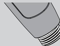
**NOTE:** Paper tab inserted to show this end of the hose assembles to hand held. Remove tab.
