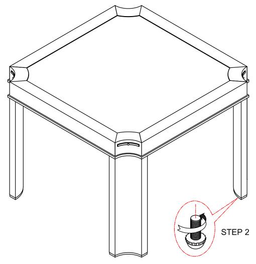
Adjust leveler if needed to level table on uneven floor.
