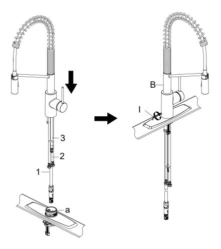
Insert the hose (1) supply lines (2) and quick connect hose (3) one by one through the hole of the base (a). Carefully insert the hoses into the base. Place the faucet assembly onto the base (a) as shown in the above figure. Secure the faucet assembly (B) by tightening the set screw with the provided hex wrench (I, Hex: 2.5 mm).
