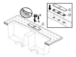
Place the escutcheon (C) and the gasket (D) on the sink. Insert the base (a) into escutcheon (C). Note: "Front" on the base (a) must face the front of the sink. The two mounting plates (b) on the base (a) must be loose and movable during the installation of the base (a). If the sink is uneven, use silicone under the gasket (D).
