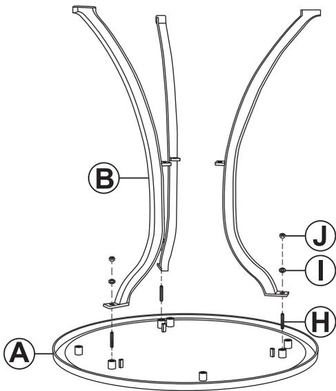
Install three Grub Screws (H) into Tabletop (A). Loosely install three Table Legs (B) using Washers (I) and Nuts (J).
