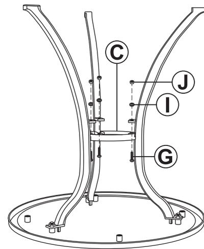
Loosely install Table Support (C) to the legs using three Bolts (G), Washers (I), and Nuts (J).
