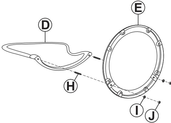
Install two Grub Screws (H) into Backrest (D). Secure the backrest to Seat (E) using two Washers (I) and Nuts (J).
