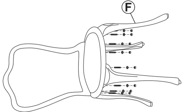
Install four Grub Screws (H) into the bottom of the seat.
