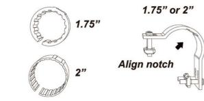
Some applications may require optional friction tape between rubber bushings for a secure, tight fit, this can be found at most local hardware stores
