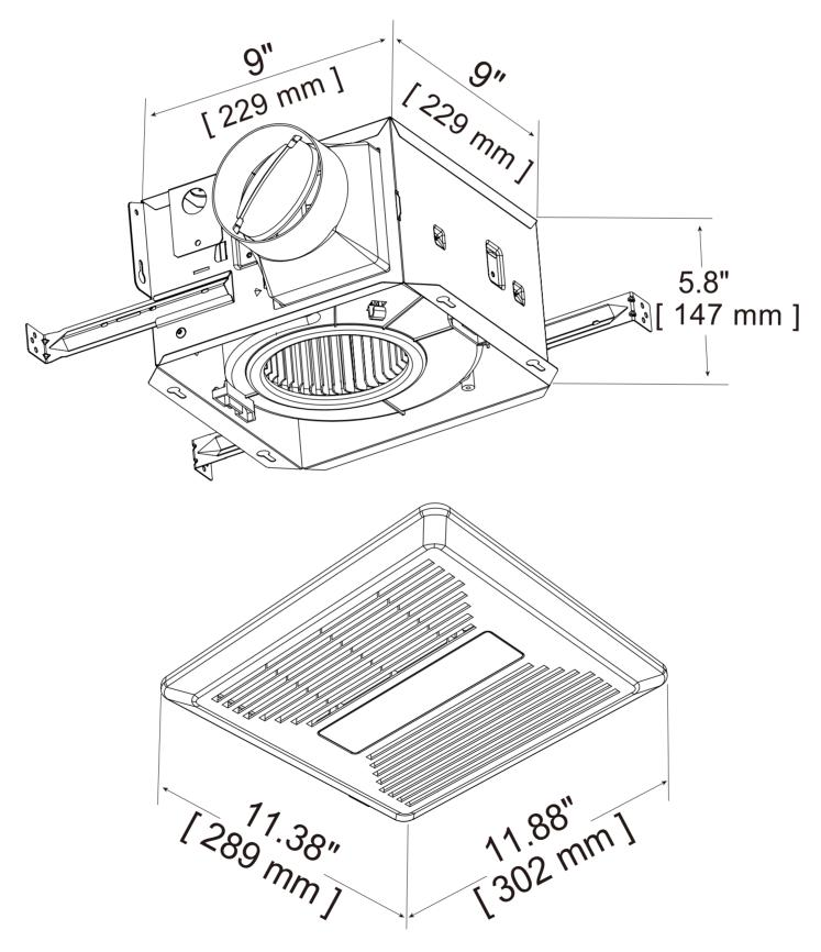
This fan can be installed to 9" - 24" between the joist or to I-joists, standard joists and truss construction.
