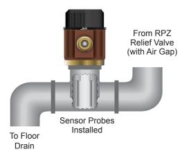
3. Unscrew the black cap to access the sensor probes. Push the two metal probes down until they touch the bottom of the pipe, then pull them up at least ¼". The ends of the sensor probes should be located between ¼" and ½ of the pipe's inner diameter from the pipe bottom. The probes **MUST NOT BE** less than ¼" from the pipe wall. Hand tighten the white plastic nuts on the probes to make it water tight.
