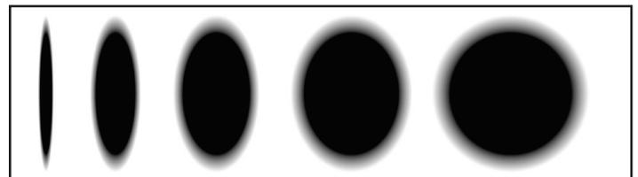
**Pattern Orientation** - A flat or semi-round spray pattern can be adjusted to any angle from horizontal to vertical by turning the Air Nozzle. Pattern is perpendicular to "ears" on nozzle. That is, when the ears are horizontal, the spray pattern will be vertical and when the ears are vertical the spray pattern will be horizontal.
