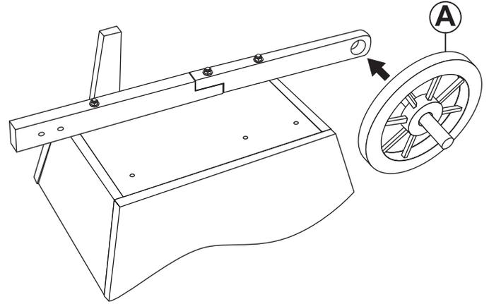
Position Wheel (A) into the hole on the front support.
