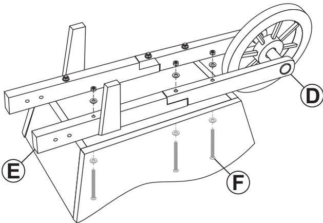
Loosely secure remaining Front Support (D) and Back Leg (E) by hand-tightening three M6x55mm Bolt Sets (F).
