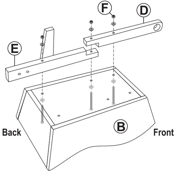
Loosely fasten one Back Leg (E) and one Front Support (D) to the bottom of Planter Box (B) by hand-tightening three M6x55mm Bolt Sets (F).
