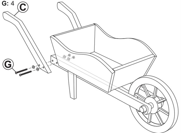
Secure one Handle (C) to the outside of a back leg using two M6x45mm Bolt Sets (G).
