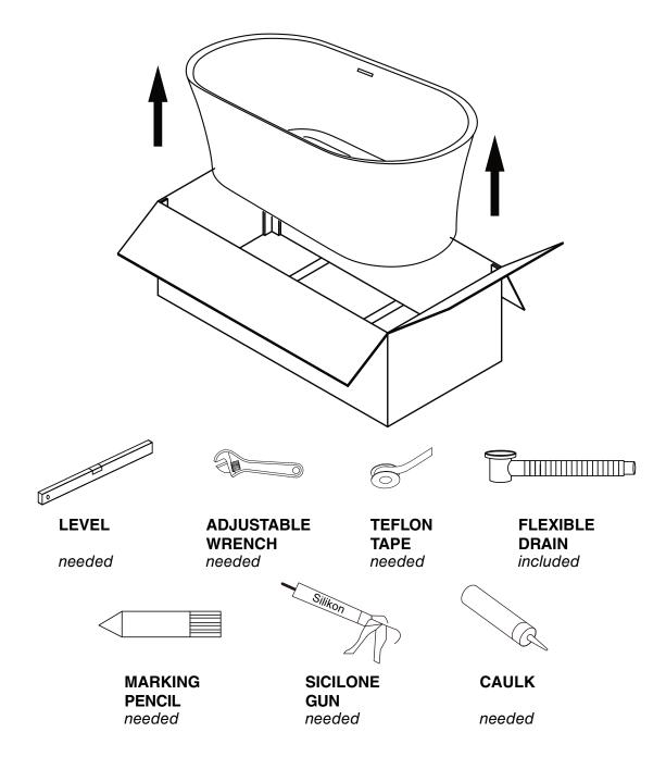
**NOTE:** THE INCLUDED FLEXIBLE DRAIN IS TO BE USED ONLY TO TEST THE BATHTUB BEFORE PERMANENT INSTALLATION. IT IS THE RESPONSIBILITY OF THE INSTALLER TO PROVIDE THE PERMANENT DRAIN ASSEMBLY.
